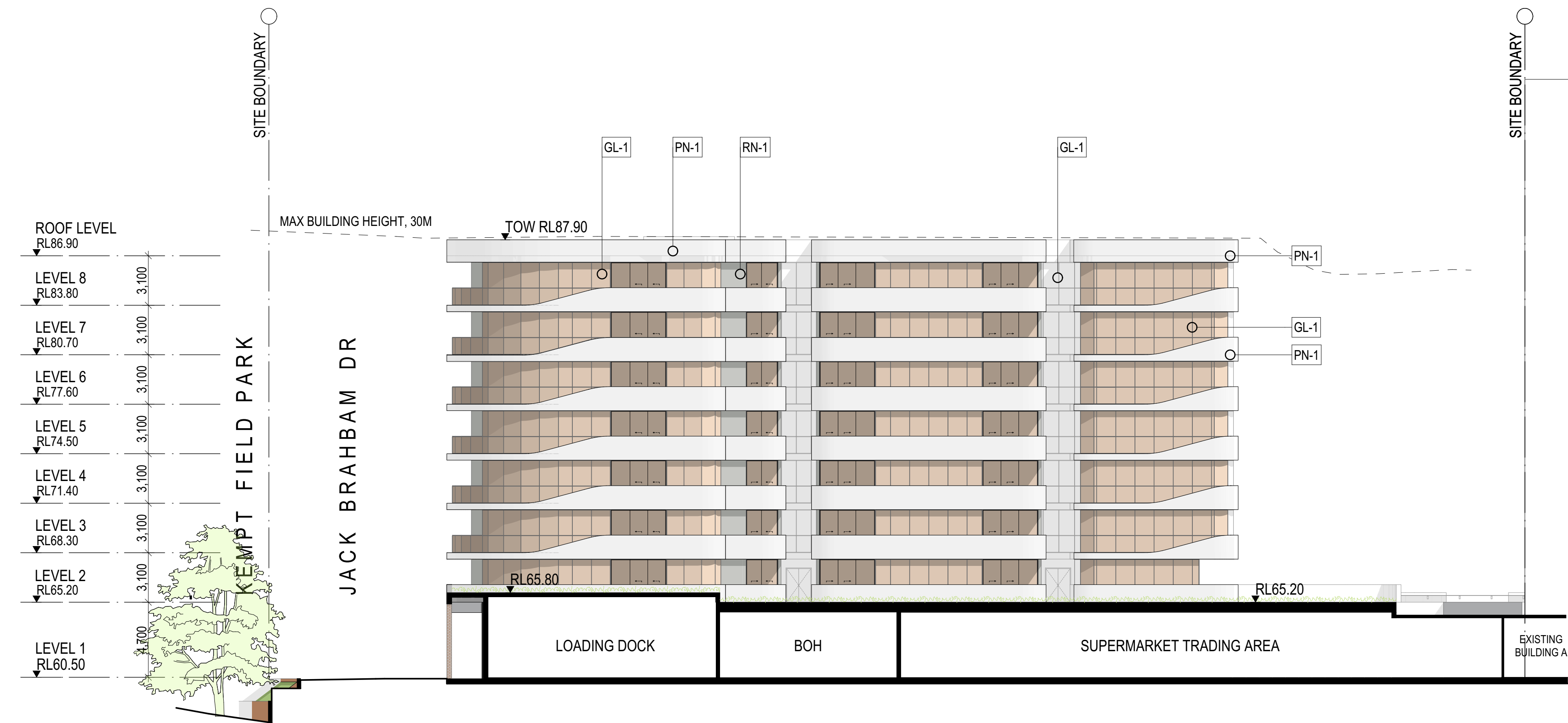
6 Building X2 - North Elevation 1:200
